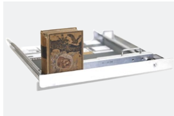
Bookmeter – a device for taking books measurements
